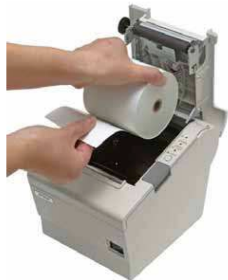
Open the lid – insert the roll – close the lid! Couldn't be easier!
